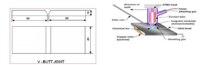
1. Prepare the edges of the work pieces to be joined to the required V shape.
